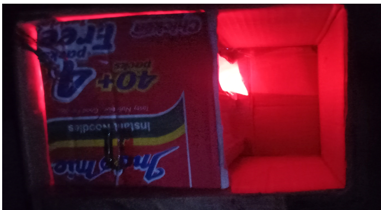
Plate 4: Phototactic Test Chamber showing red LEDs light.
